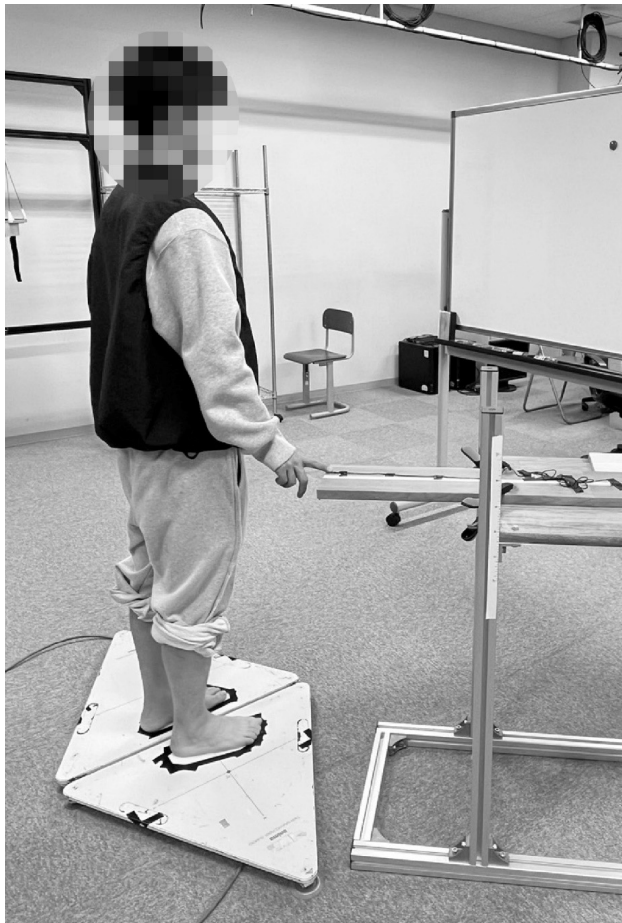
Figure 1. Experimental setup. This figure represents a measurement in the quiet standing position under the light-touch condition. Under this condition, the participants placed the tip of their dominant index finger on a load cell.
